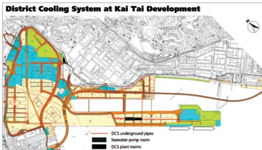
地圖顯示啟德發展區區域供冷系統的服務範圍和地下水管網絡 A map shows the service area and underground water-piping network of the District Cooling System at Kai Tak Development
