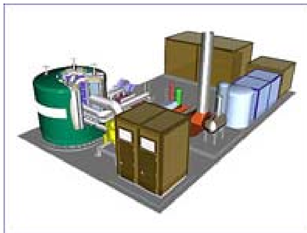
Figure 7-6: FCE 1 MW MCFC Power Plant
