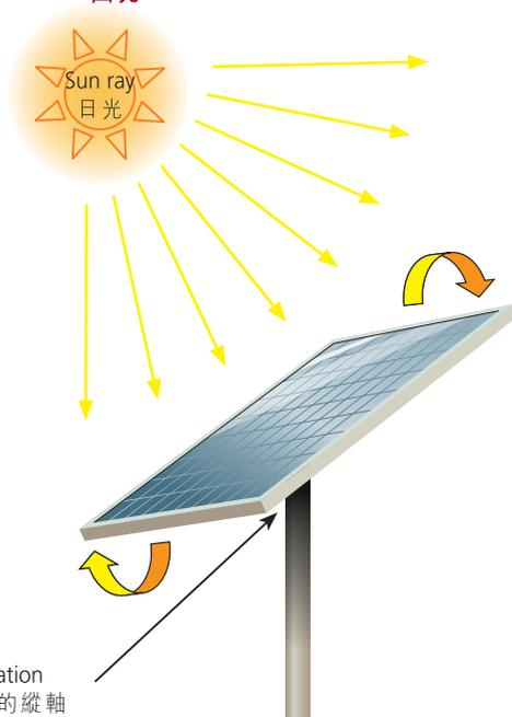
Figure 2: Illustration of a typical single-axis tracker rotating the PV panel gradually from east to west during the day
