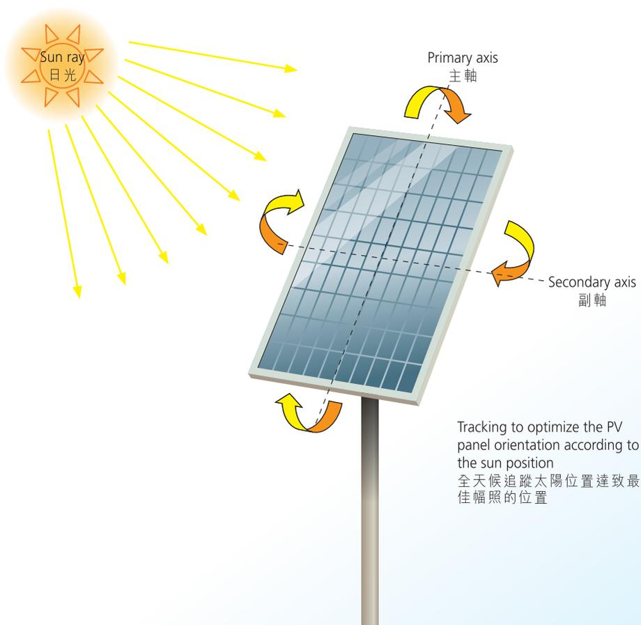
Figure 3: A typical two-axis tracker rotating the PV panel around 2 axes, i.e. one axis for inclination with the ground and the other axis for orientation along east-west direction
