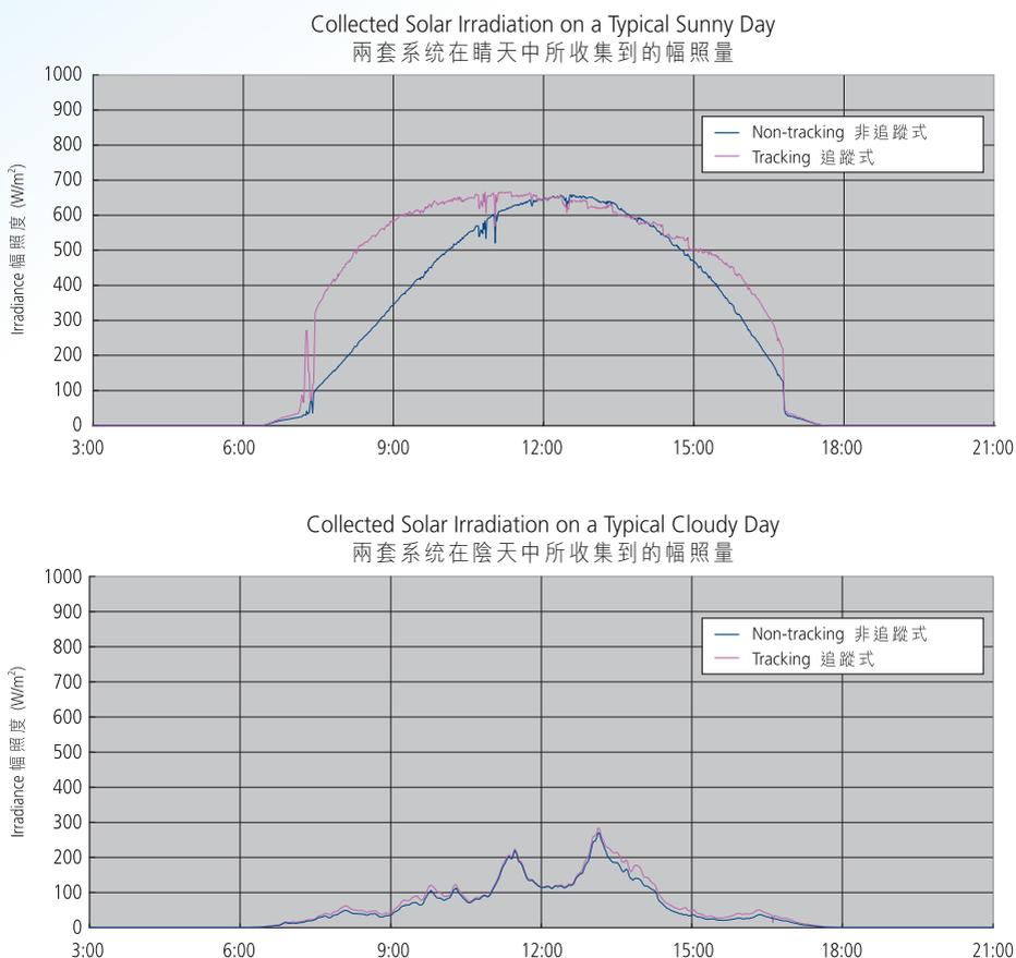
Figure 4: Collected solar irradiation on a typical sunny day and a typical cloudy day in the monitoring period
