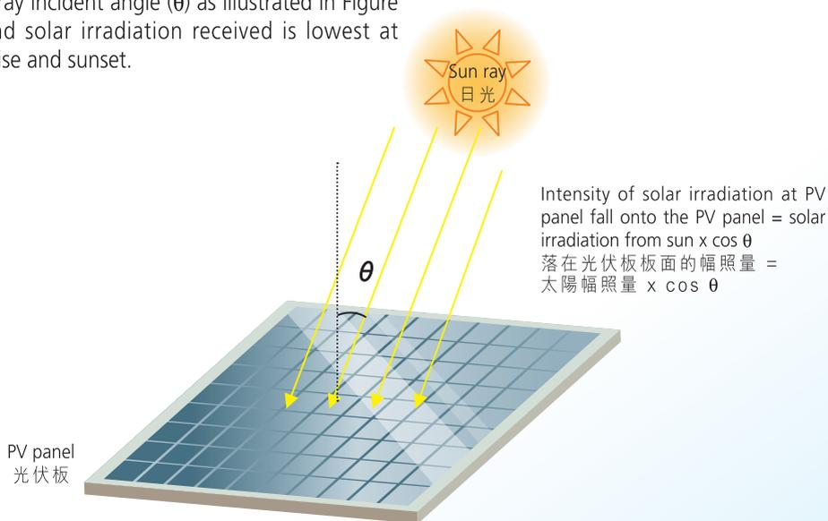
Figure 1: Solar irradiation fall onto the PV panels is related to the cosine of the sun ray incident angle ( $\theta$ )
