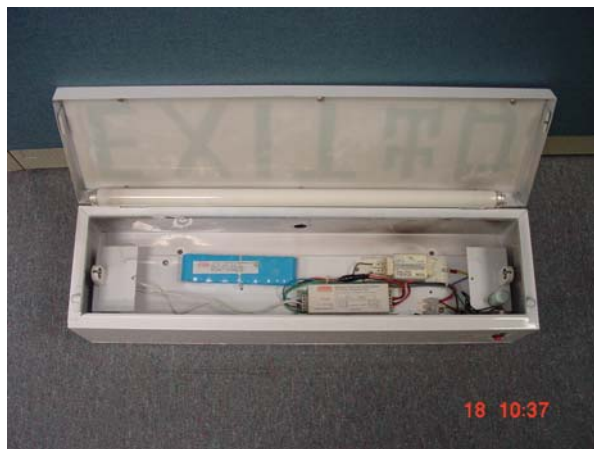
Fig. 3: Internal components of a conventional EXIT sign
