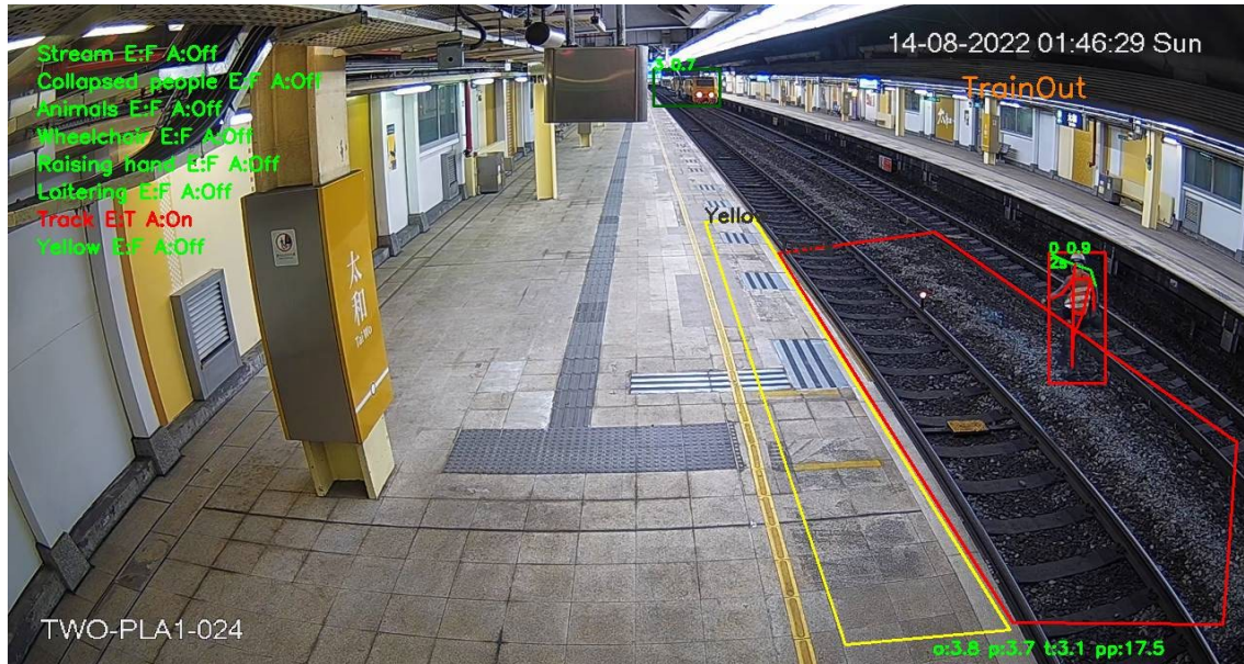
Figure 5 Illustration of the detection of person on track at East Rail Platform
