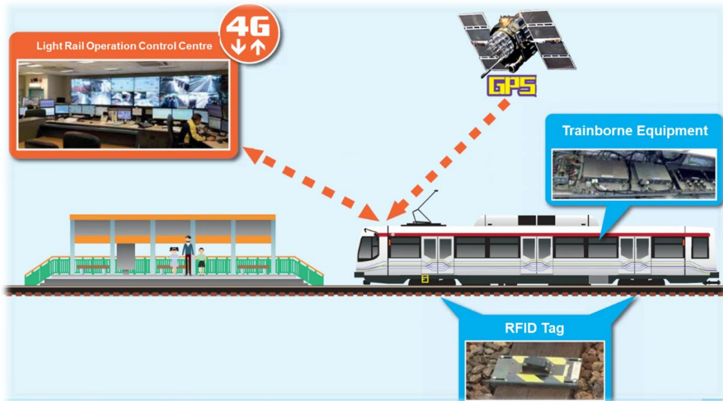
Figure 8 Integration of RFID and GPS signal for iSPS
