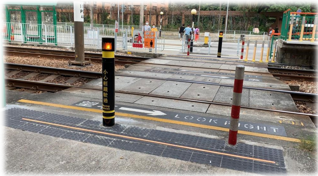
Figure 10 Smart Bollard at pedestrian crossings
