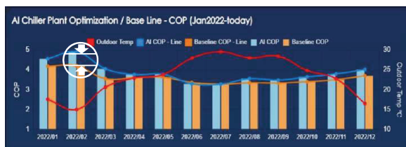
Figure 7(a) Improvement of COP Using AI
