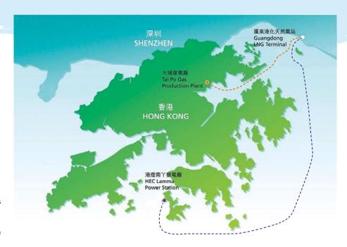
· 海底管道往大埔煤氣廠 Submarine Pipeline to Tai Po Gas Production Plant
