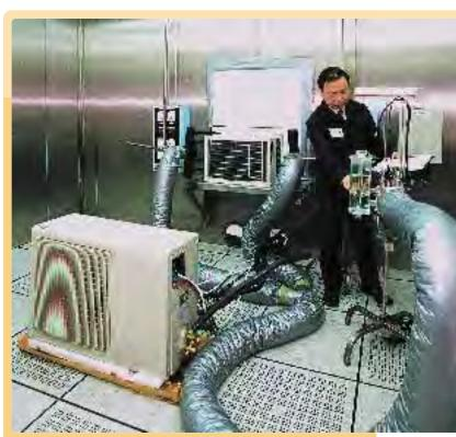
香港科技大學實驗室內正進行冷氣機能源效益標籤測試。 Testing of air-conditioners for energy efficiency labelling at a laboratory in the Hong Kong University of Science and Technology.
