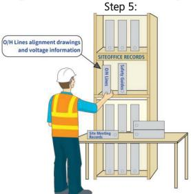
Working party should ensure all information about the O/H lines (e.g. alignment, distance from ground, voltage of the O/H line) and safety advice from the electricity supplier are made available for site personnel (e.g. supervisors, signallers, plant operators and workers), and working party should retain site meeting records described in Section 6.2.4 for inspection upon request by the Director.
