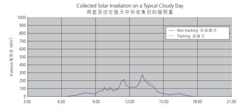
Figure 4: Collected solar irradiation on a typical sunny day and a typical cloudy day in the monitoring period 圖四: 兩套系統在睛天和陰天所收集到的幅照量比較
