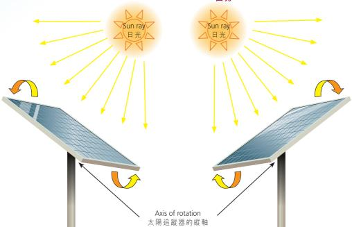
Figure 2: Illustration of a typical single-axis tracker rotating the PV panel gradually from east to west during the day 圖二:示意圖顯示典型單軸太陽追蹤器在日間按太陽位置漸進地把光伏板的面向由東方轉動至西方
