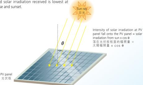
Figure 1: Solar irradiation fall onto the PV panels is related to the cosine of the sun ray incident angle (θ) 圖一:落在光伏板板面的幅照量按入射角的餘弦而定
