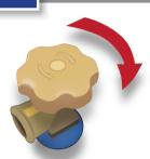
1. Close the cylinder valve completely by turning it clockwise.
