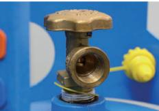
2. Check the cylinder valve and its inner thread, and ensure there is no obvious damage.
