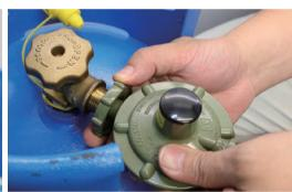
3. Hold the regulator firmly with one hand and turn its handwheel anticlockwise with another hand until tight interlock with the cylinder valve is secured.
