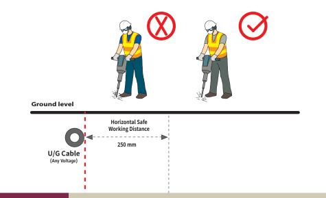
Minimum horizontal safe working distance between any U/G cable and the point where hand-held power tools are used for breaking out paved concrete surface.
