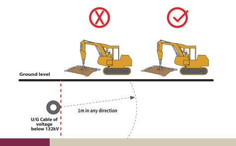
Minimum safe working distance between U/G cables of voltage below 132 kV and the point where mechanical excavators are used.
