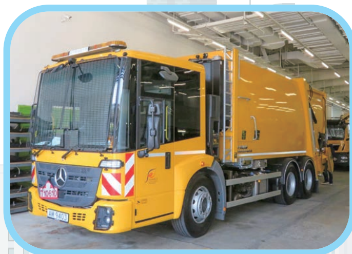
The first batch of low-entry refuse collection vehicles procured by the FEHD in 2019 (with the Econic chassis of Mercedes-Benz and refuse hopper of FAUN Variopress)
