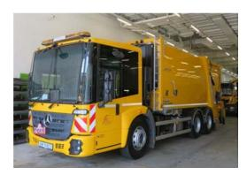
The major difference between the chassis of a traditional truck and that of a truck with low-entry is the design of the driving cab. The two major benefits of a low-entry design are as follows:
