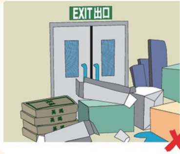
A huge pile of construction materials is stacked at the fire escape, causing obstruction.
