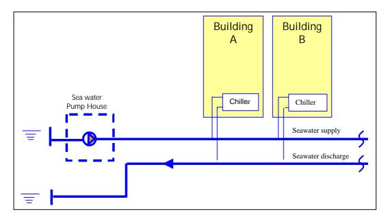
For a building served by Central Seawater Scheme, its air conditioning system uses seawater for cooling the chiller condenser. A dedicated central seawater supply system distributes seawater from the sea to the user building. The rejected warm seawater from the chiller condensers will be discharged to the sea through another dedicated outfall pipe. For this scheme, a central seawater pump house and a central distribution pipeline network are required.
