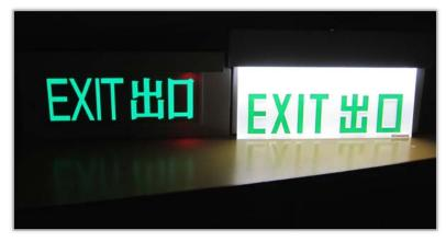
Figure 2 – Photo of tested LEC exit sign (left) and LED exit sign (right)
