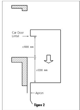
5.14.3 The means shall be capable of performing as required in Clause 5.14.1 without assistance from any lift component that, during normal operation, controls the speed or retardation, or stops the car, unless there is built-in redundancy and correct operation is self-monitored.
