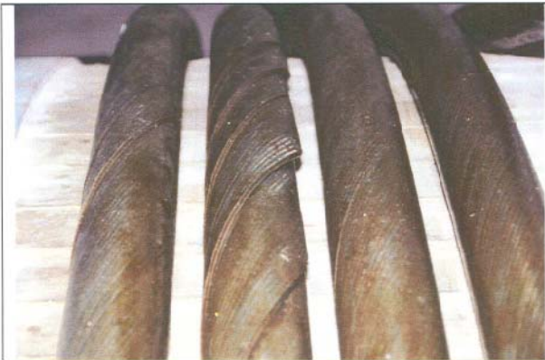
Fig. 14: Structural problems of the carrying ropes in the outer layer of z-wires
