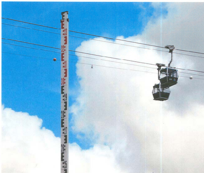
Fig. 5: Measuring assembly for the observation of the peak-to-peak swings that the ropes perform during acceleration and deceleration phases (conducted on 26. 6. 07)
