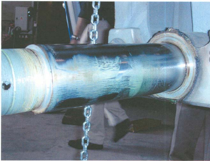
Fig. 4: The suspension shaft was in perfect condition, more than sufficient lubricant was present.
