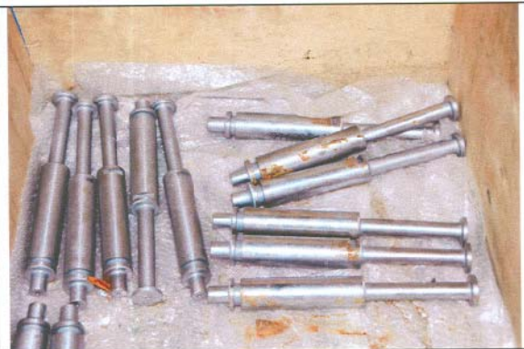
Fig. 11: Even the new axles of the connection of suspension and cabin show traces of rust.
