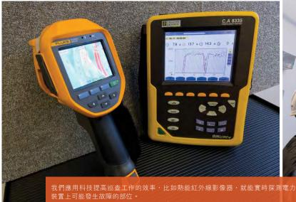
Thermal imagers are examples of how we apply technology to make inspection work more efficient. The device can identify potential faults on
