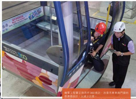
感應器設計,以減少出錯。 EMSD has been working with Ngong Ping 360 to enhance the design of cabin door locking sensor to minimise false tripping.
