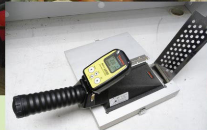
在簡介會上示範表面輻射污染探測器的操作方法。 The operation of Surface Contamination Monitor was demonstrated in briefing sessions.
