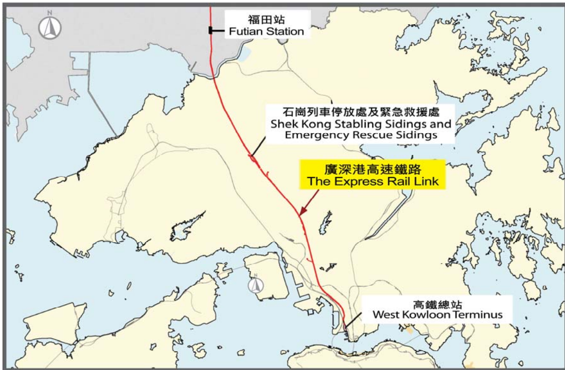
Fig. 1. Alignment of the Hong Kong section of the Guangzhou – Shenzhen – Hong Kong Express Rail Link
