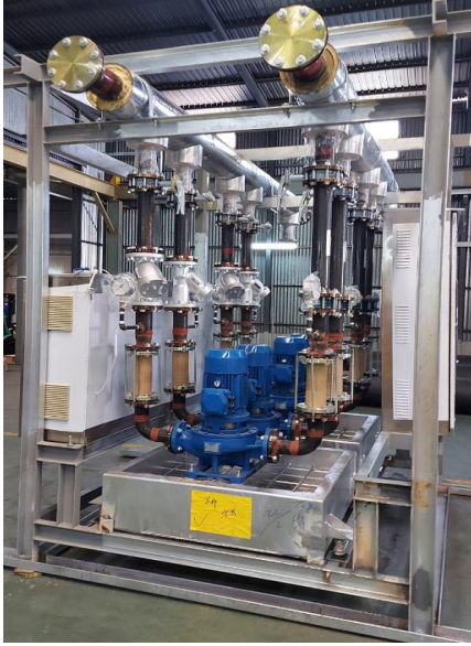
Figure 2. Off-site prefabrication of chilled water pump set
