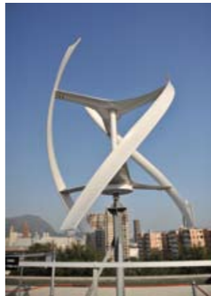
豎軸(直立式)風力發電機(風車) Vertical axis wind turbine
