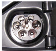
IEC 62196 Type 2 Vehicle Inlet
