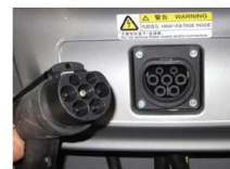
GB 20234.2 AC Vehicle Connector and Vehicle Inlet
