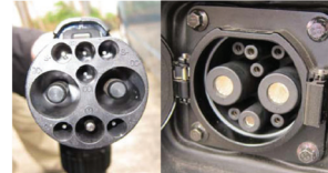
GB 20234.3 DC Vehicle Connector and Vehicle Inlet
