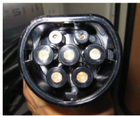
IEC 62196 Type 2 Vehicle Connector
