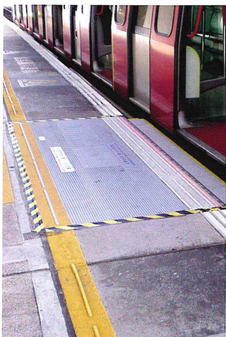
羅湖車站試驗自動伸縮月台踏板，以加強乘客安全。 Mechanical gap fillers being tested at Lo Wu Station to enhance passenger safety.
