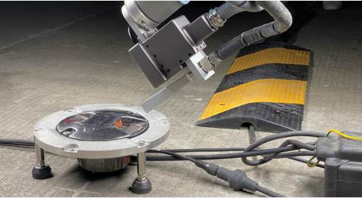
(左)機場跑道助航燈自動維護機械人可自動偵測和清潔跑道燈，騰出手處理其他工作。該創新方案大幅提升維修效率，同時確保跑道安全。 (右)去年11月，立法會議員到訪機電署總部，透過現場示範了解機場跑道助航燈自動維護機械人的應用情況。 (Left) The Autonomous AGL Cleaning and Inspection Robot can automatically detect and clean the airfield ground lights, freeing up manpower for other tasks. This innovative solution significantly enhances maintenance efficiency while ensuring runway safety. (Right) In November last year, Legislative Council members visited the EMSD Headquarters and learned about the application of the Autonomous AGL Cleaning and Inspection Robot through an on-site demonstration.
