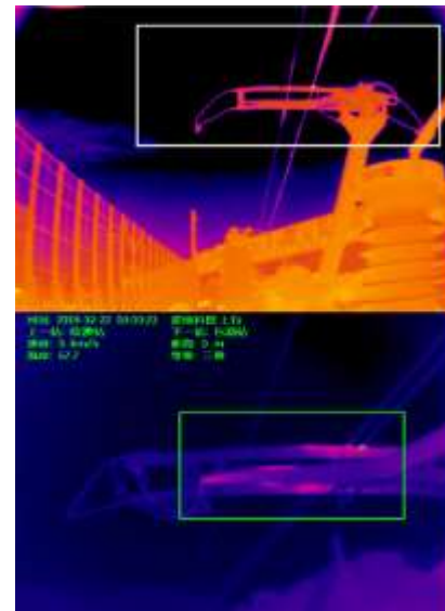
Arcing and High Temperature Detection at Section Insulator
