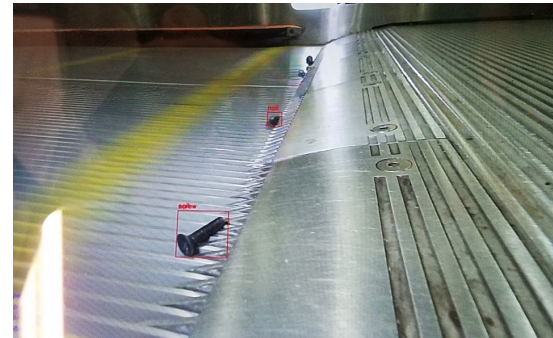
Figure 7(d): Detection of small objects in escalator
