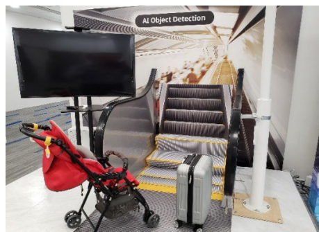
Figure 7(e): Detection of bulky objects in escalator
