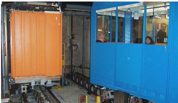
A multi-dimensional transport system that combines lift and tramway technologies
