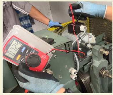
Measuring holding voltage of the brake coil
