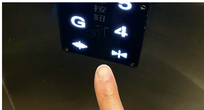
Contactless buttons utilising capacitive sensing technology
