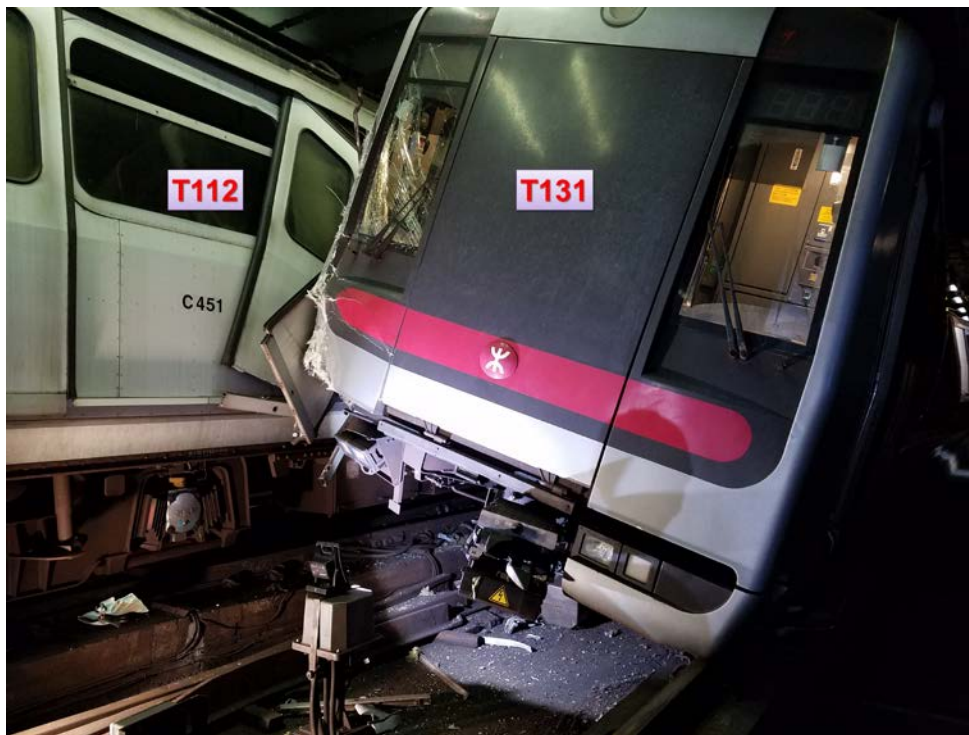
Figure 1: Condition of the trains after collision
