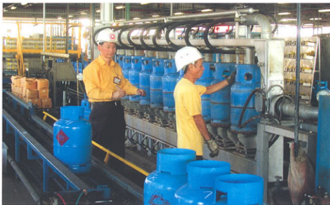
Checking for leakage of LPG cylinders
