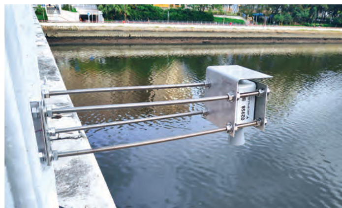
政府物聯通的防洪監測傳感器 Flood monitoring sensor of the GWIN
