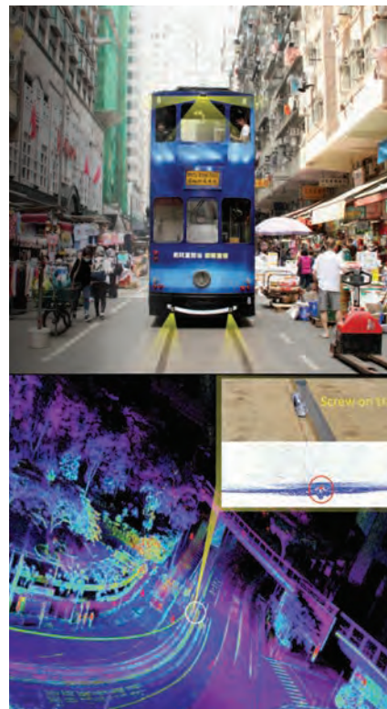
預防電車脫軌及碰撞系統 Tramway Derailment and Collision Prevention System
