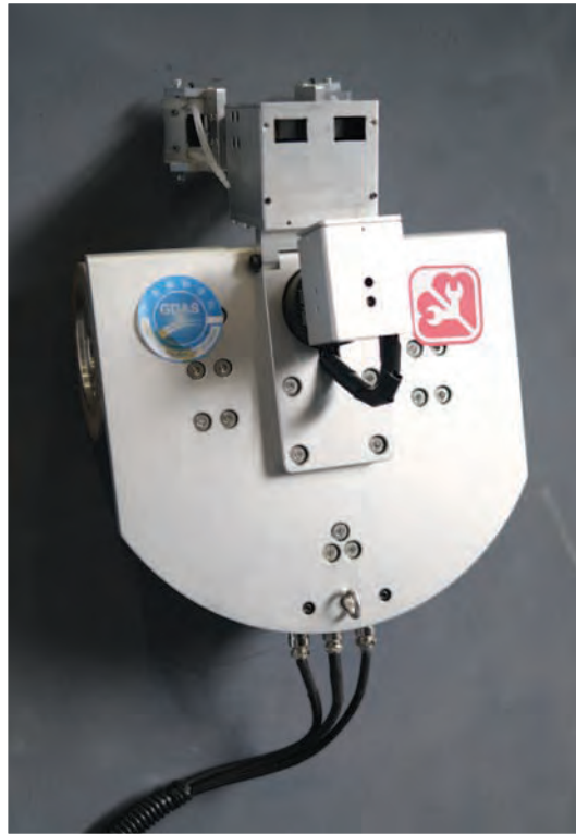
智能液化石油氣缸車檢測機械人 LPG Tank Inspection & Data Analysis with Intelligent Tanker Robot
