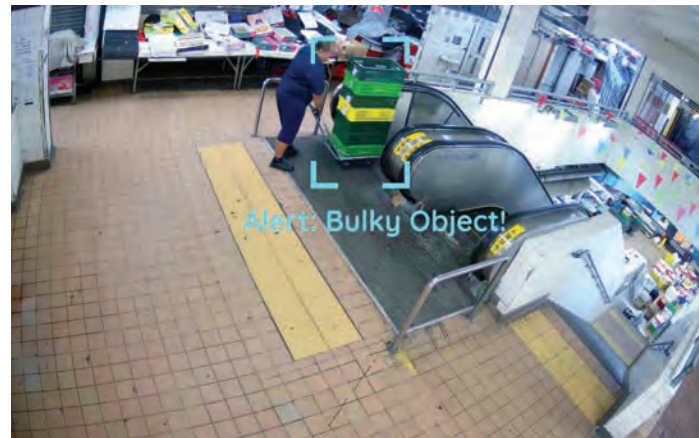
人工智能影像分析系統監察香港街市的自動梯運作 AI Video Analytics System for Escalator Monitoring in Wet Markets of Hong Kong
