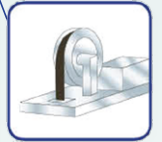
3. Install an ascending car overspeed protection device
