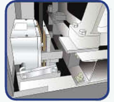
2. Install an unintended car movement protection device on the brake system
