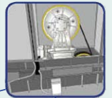
2. Install an unintended car movement protection device on the brake system
