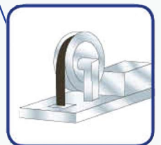
3. Install an ascending car overspeed protection device
