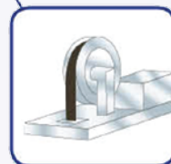
3. Install an ascending car overspeed protection device
