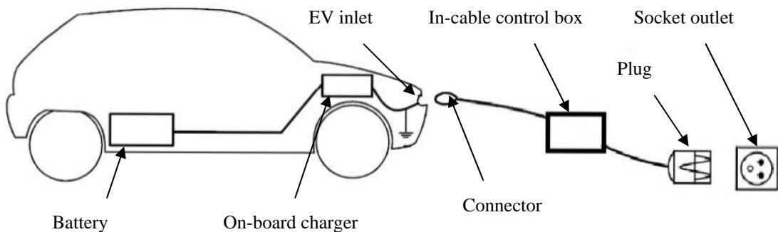
Mode 3 - Use of a dedicated socket outlet where control pilot cable permanently connected to ac source
