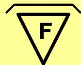
Symbol for minimum distance from lighted objects, if applicable, for luminaires which might otherwise overheat the lighted objects due to for example the applied lamp type, the shape of the reflector, the adjustability of the mounting means or the location of mounting as indicated in the installation instructions
