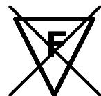
Symbol for suitability for mounting in/on combustible surface when thermally insulating material is used to separate the luminaire from the surface
