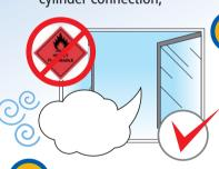
All LPG blow torches must be used, replaced and kept in a well-ventilated location away from inflammable materials;
