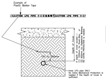
Note: Even with mechanical protection, depth of cover of U/G LPG pipes cannot be smaller than 100 mm
