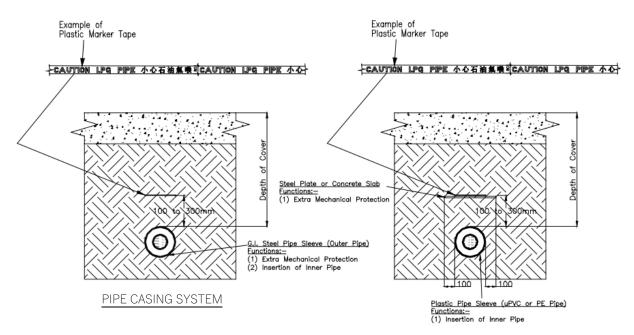
PIPE CASING SYSTEM + STEEL PLATE OR SLAB
