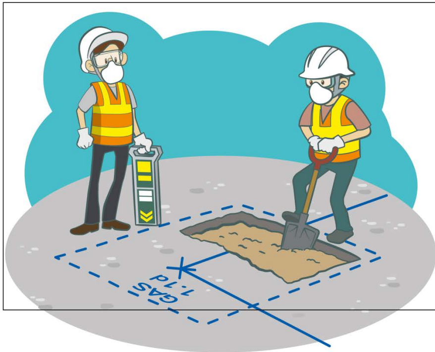
Image 5 - Digging of trial holes by use of hand tools
