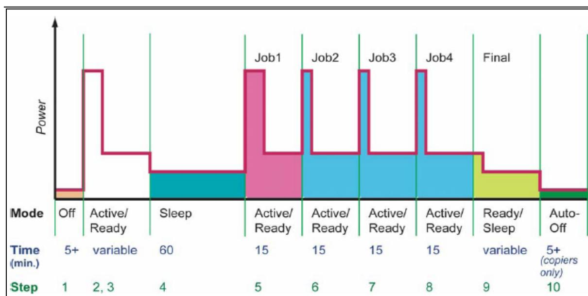
Figure 1 shows a graphic form of the measurement procedure. Note that products with short default-delay times may include periods of "Sleep" within the four job measurements, or Auto-off within the "Sleep" measurement in the Step 4. Also, print-capable products with just one "Sleep" mode will not have a "Sleep" mode in final period.
