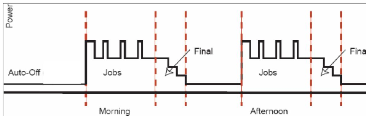
Figure 2 shows a schematic example of eight-ipm printer that performs four jobs in morning, four jobs in afternoon, has two “final” periods and an Auto-off mode for the remainder of the workday and all of the weekend. An assumed “lunchtime” period is implied but not explicit. The figure is not drawn to scale. As shown, jobs are always 15 minutes apart and in two clusters. There are always two full “final” periods regardless of the length of these periods.
