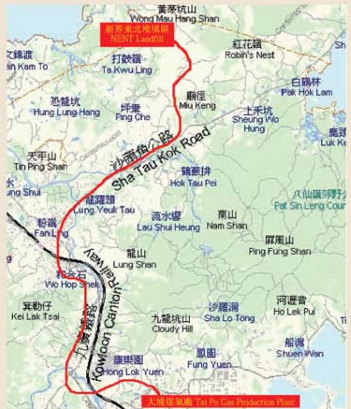
Figure 4 Landfill Gas Pipeline Route Map
