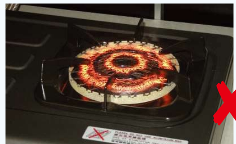
When "energy saving wire mesh" is used, the burner flames turn yellow.
