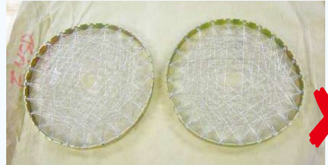
Using "energy saving wire mesh" will increase the emission of carbon monoxide.
