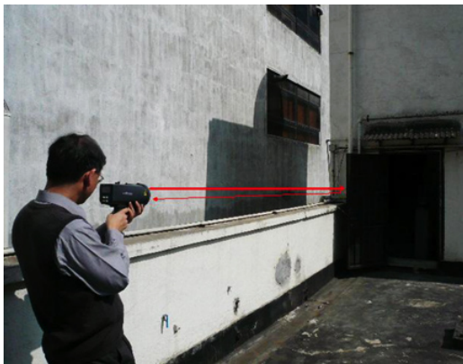
Figure 2: Remote gas detector being tested
