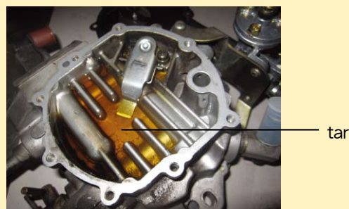
Figure 2: The LPG that cannot be vaporised during vaporisation is called tar (the brown liquid) and would accumulate in the vaporiser. An excess of tar would cause the vehicle to stall while running.
