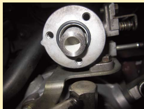
Figure 3: The idle speed fuel filter would filter out the residues during the process of vaporisation. If not properly maintained, it could cause stalling during idle speed.
