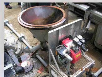
Main burner specially made for special pyrotechnics effects
