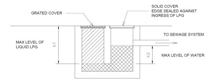
$h_1$  is the required depth of the weir to prevent passage of liquid LPG through the trap to the sewage system. It is calculated based on that if  $h_2$  is filled with water up to the bottom of the outfall pipe and  $h_1$  is filled to grade with liquid LPG, the water in  $h_2$  can balance the LPG in  $h_1$  and thus in a no flow position.
