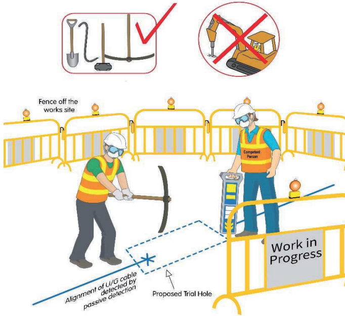
Fig 3.4 - Trial hole Excavation (Step 1)
